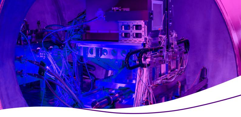
PIMEGA-540D is a photo counting detector based on pixelated semiconductor sensors assembled over Medipix3RX ASICs. It brings together important features for direct X-Ray detection such as superior signal-to-noise ratio, single-photon counting, and high detection efficiency.
